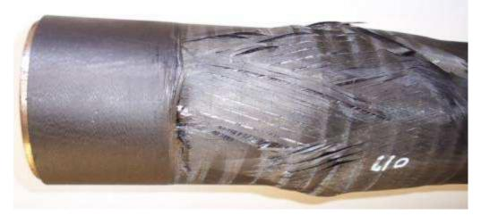
Hybrid laminate to reduce confinement of slender motors at elevated temperatures
